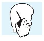
otherwise, the radio operates normally. Lift it to about 15 cm from your face with the speaker beside your ear and the bottom of the radio beside your mouth as shown. Press and hold the PTT key each time you speak, as described above.
